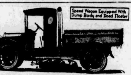
Speed Wagon Equipped With Dump Body and Road Floater
