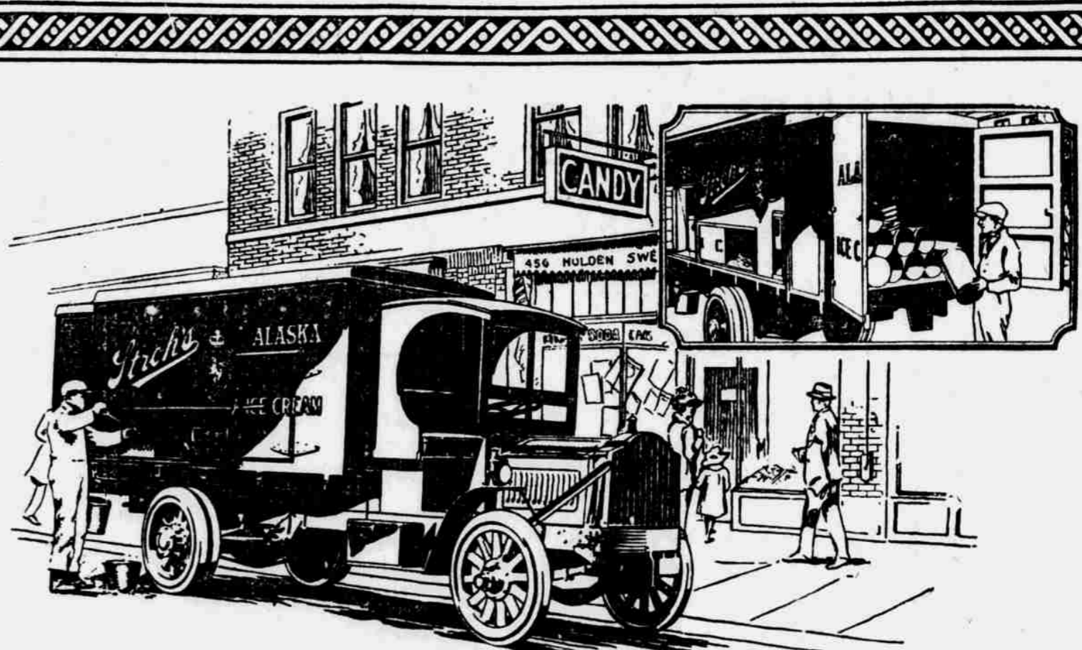
The latest in Ice Cream bodies—a special-bodied Packard with separate compartments for the cream—salt—ice and empty cans. No BRINE to drip and ruin the truck's working parts.
