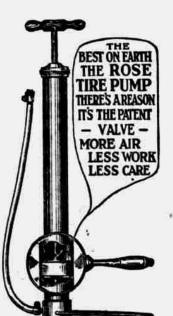
The Rose tire pump pumps more air because it does not get its air supply around the cupped leather as do other pumps, but instead through the patent valve. Therefore, the cupped leather never leaves the walls of the cylinder and the instant the plunger starts on the downward stroke the compression starts. The supped leather is long lived because it holds but one position and is not continually opening and closing with each upward and downward stroke of the plunger.
