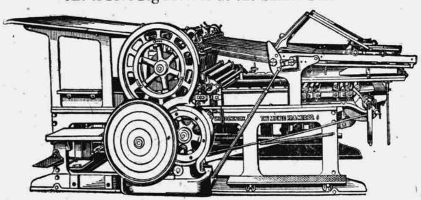
This is but one of a battery of five | largest of which accomodates a form | with an automatic feed delivery, with big Miehle cylinder presses, the of 68-inch type space. It is equipped an electric derrick for raising heavy paper stock to the feed board.
