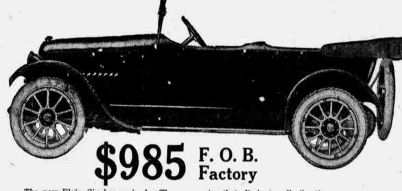
The new Elgin Six has arrived. The new motor that eliminates all vibration. The new Elgin is more powerful and is finished better than ever. Wheel base 116 inches, Bogg Beck clutch, full floating axle, forty-eight-inch full cantiliver springs, double cowl body, neverleak top, Jiffy curtains. Large over-sized tires, 33 by 4.
