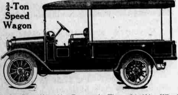
3-Ton Speed Wagon Engine Size, 4 1/2 x 4 1/2. Pneumatic Tires, 34 x 4 1/2. Wheel Base, 121 inches. Price $1,000 f. o. b. Factory.
