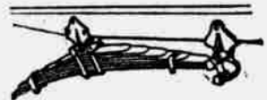
True cantilever springs 50 1/2 x 2 inches. Long and resilient, made of seven leaves with two top leaves of special Tungsten steel, the major shock of every road is absorbed before it reaches the body of the car.
