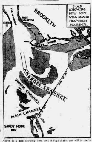
Above is a map showing how the new steel net, now being made aboard the old monitor Amphitrite at the Brooklyn navy yard, will guard New York harbor from the invasion of submarines. The net is constructed of heavy steel cable and cross-sections
