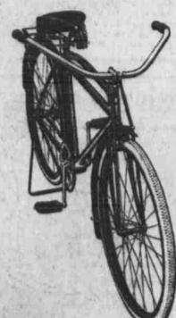
It has a 20-inch Frame with Coaster Brake. Motor Bike Handle Bars, Eagle Diamond Saddle, Motor Bike Pedals, Motor Bike Grip, Luggage Carrier Holder, Folding Stand, Front and Rear Wheel Guards, Truss Frame and Front Fork.
