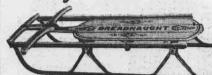
No. 132 S Dreadnaught Steering Sled—i5x14x8 \(\frac{1}{2}\)—weight 12 lbs. each. Stamped steel knees. Best crucible spring steel T-shaped runners, so curved in front as to give a maximum length of steering surface. Steering bar works perfectly, the sled responding instantly to slightest bend in steel runner without retarding speed of sled a particle. Gear and runners finished in red chamel. Top of Rock Elm, beautifully painted and decorated
