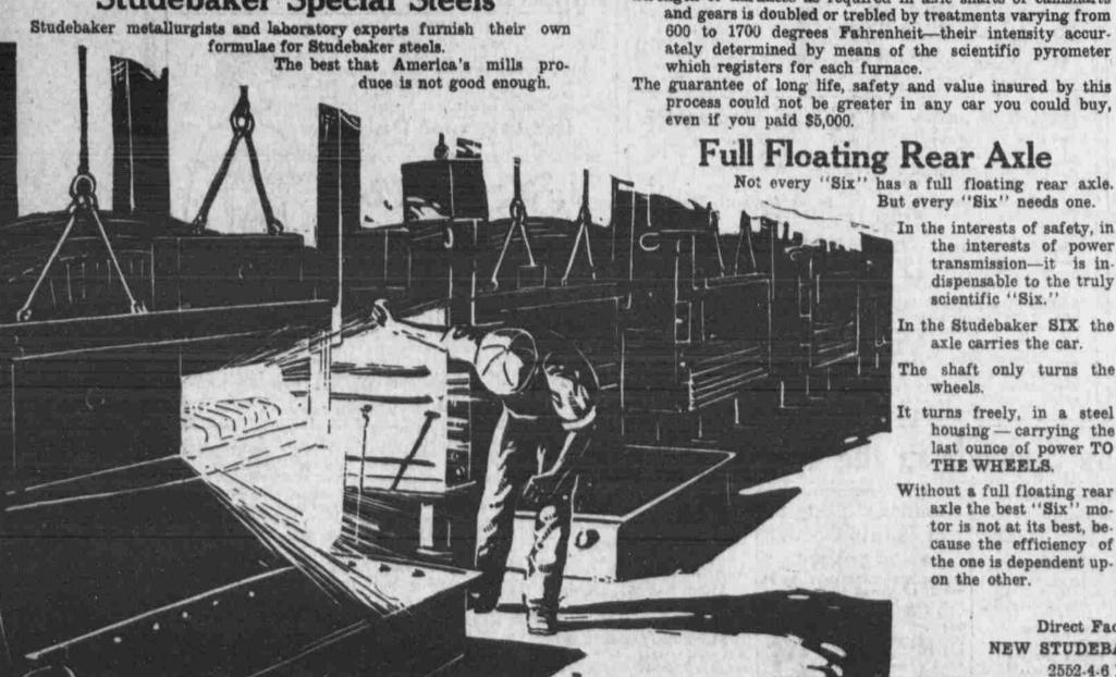
The steels must be made on special Studebaker specifications. Then these High Chrome Nickel and High Chrome Vanadium steels must show, under test, an ultimate strength of 150,000 pounds to the square inch.
