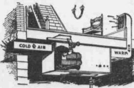
Showing how cold outside air is passed over an AMERICAN Indirect Radiator and warmed to 70 degrees before it enters the room Air of rooms is changed 2 to 4 times per hour.
