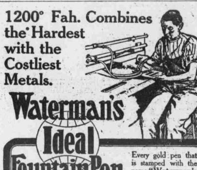
Every gold pen that is stamped with the name "Waterman's Ideal" is tipped with two little pin - head particles of selected iridium. Under an automatic blower system, the heat is applied to each individual pen blank and
