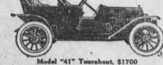
Model "41" Tourabout, $1700 Detachable Tonnage. Motor 4 1/2 x 4 1/2. Unit power plant. 110-inch wheel-base. Tires 34 x 4.
