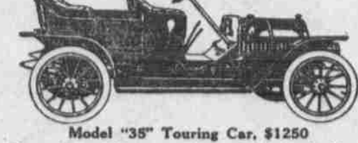
Model "35" Touring Car, $1250 Motor 4 x 4. Unit power plant. 105-inch wheel-base. Tires 32 x 3 1/2.
