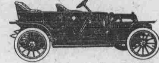
Model "35" Convertible Torpedo, $1250 Motor 4 x 4. Unit power plant. 105-inch wheel-base. Tires 32 x 3 1/2. Front doors and panels, $40 extra.
