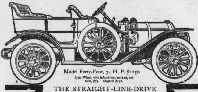
Power cannot be carried around a corner without great loss, due to friction. In the ordinary automobile much energy is wasted in transmitting the power from the engine to the rear axle through universal joints, or, in other words, around corners.
