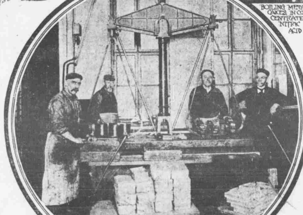
THE BEAM SCALES ON WHICH ALL DEPOSITS ARE WEIGHED
