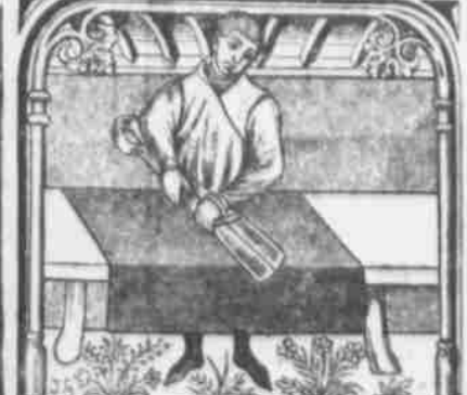
In an old French window of the fifteenth century is preserved a record of an ancient custom—the method used by the cloth-sherers. It shows how the cloth was spread upon a table and its nap removed by great scissors made like pinchers.
