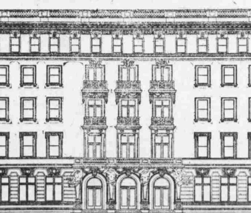
Harney Street Elevation from the Plans of Fisher & Lawrie, Architects, That Have Been Adopted by the Board of Directors.—The Building Will Be Five Stories High, 132 Feet on Harney and 157 feet on Seventeenth.
