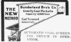
fixed screen into the wagons. The teamster controls the flow of the coal by means of a lever and the law of gravitation, together with the automatic screening device attached to the pockets, carries the coal, cleaned of all dust and dirt, into the wagons.
