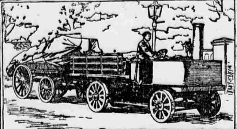
MOTOR-TRUCK WITH TRAILER CARRYING FOURTEEN TONS, ONE OF THE PRIZE WINNERS AT THE LIVERPOOL TRIALS.
