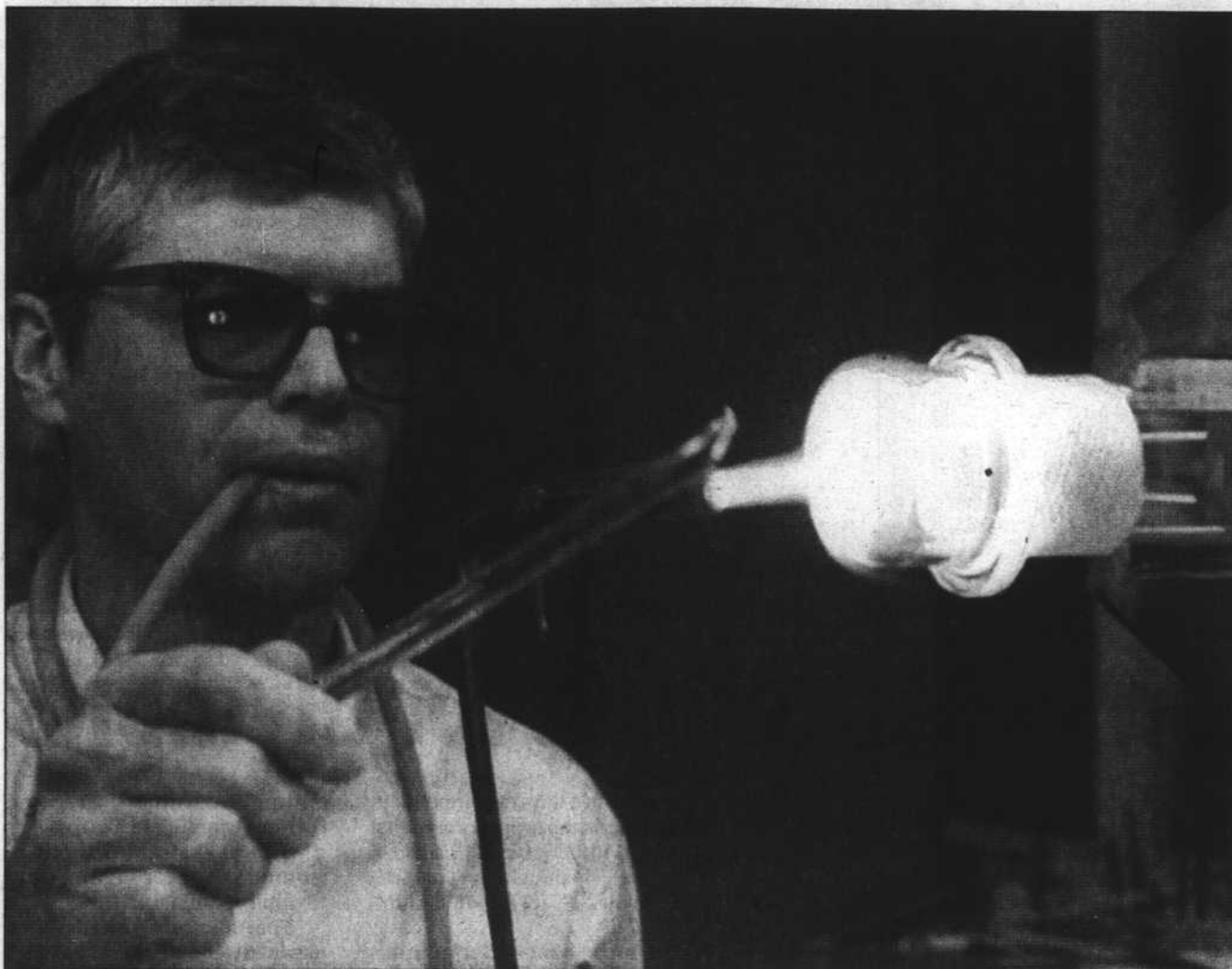
While blowing air into a plastic tube to keep a molten-glass cylinder from caving in, Hadrian Duke gives shape to laboratory glassware. Duke was hired this fall as UNL's scientific glass blower.
