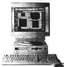
Macintosh Performa 6214CD 8MB RAM/1GB hard drive, PowerPC 603 processor, CD-ROM drive, 15" color monitor, keyboard, mouse and all the software you're likely to need.
