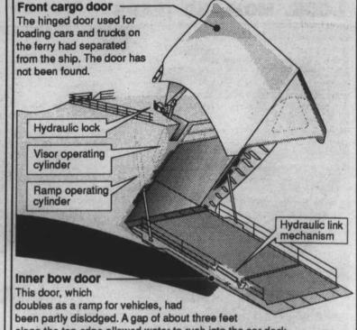
along the top edge allowed water to rush into the car deck.
