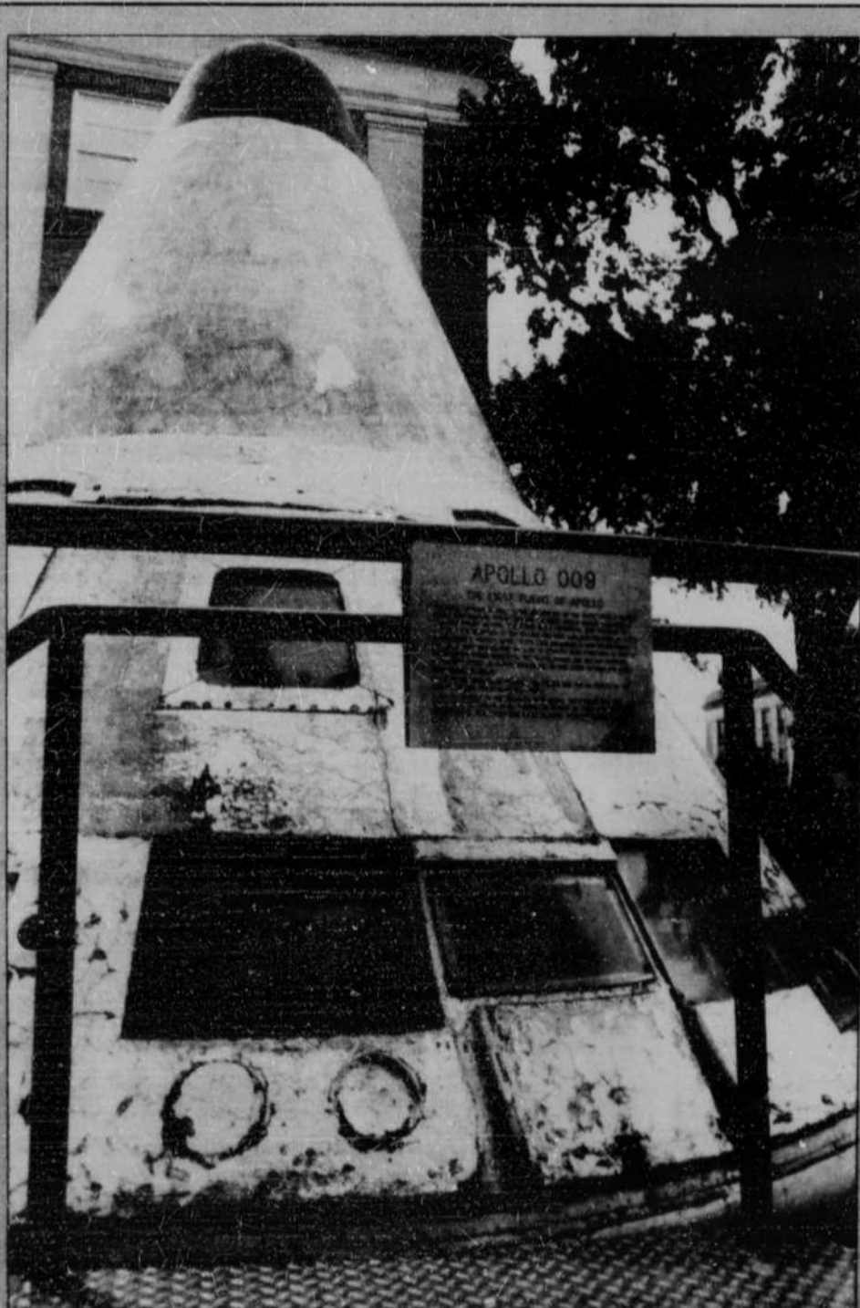
Eighteen years of Nebraska weather have caused serious damage to the historic Apollo 009 space module on display in front of Morrill Hall.
