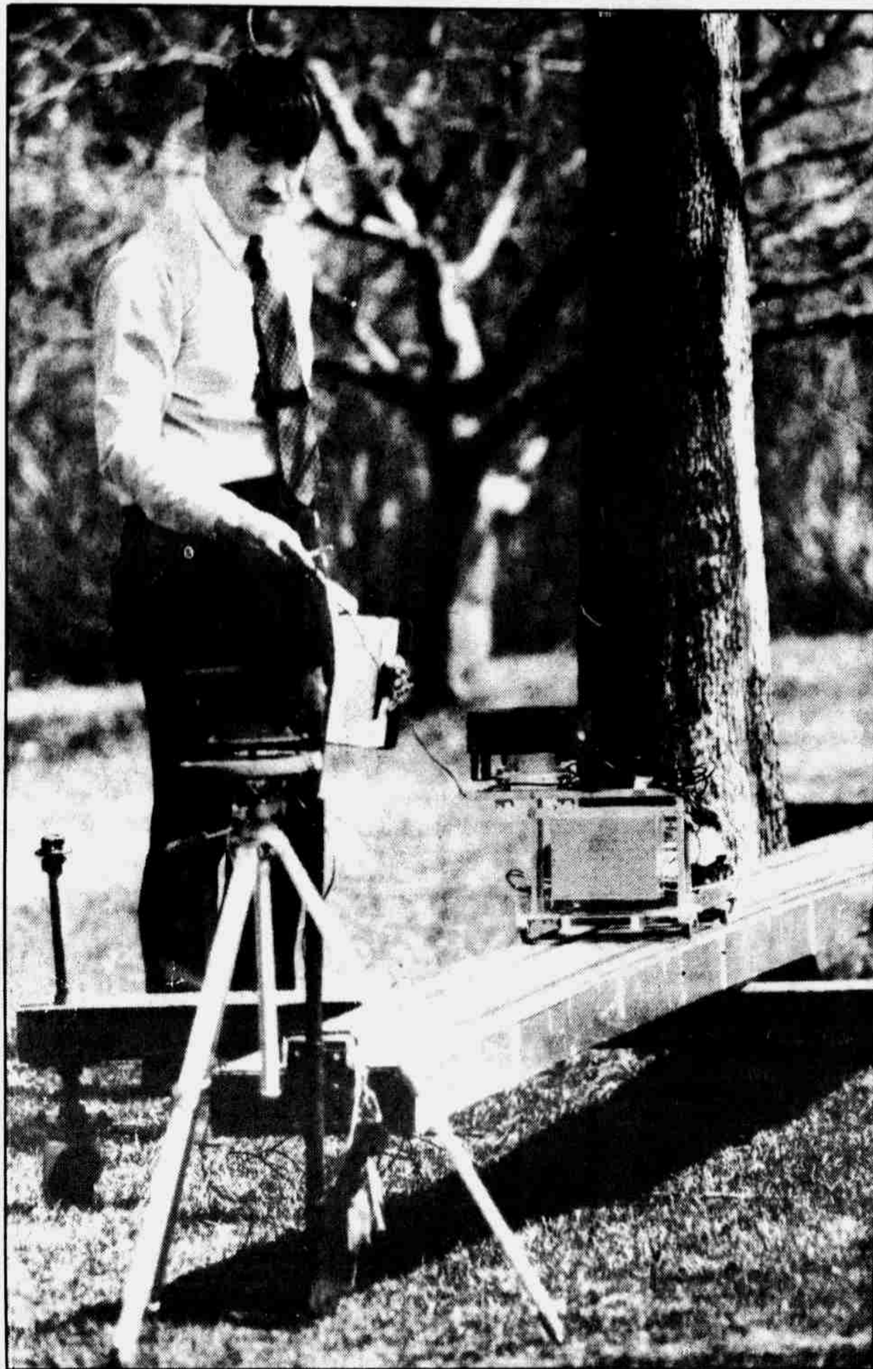
Photo by D. Eric Kircher Robert Youngberg, director of the UNL Solar Office, watches a test device that measures solar energy filtering through tree canopies. The information will be used to make recommendations on the best trees to plant to block and admit solar energy.
