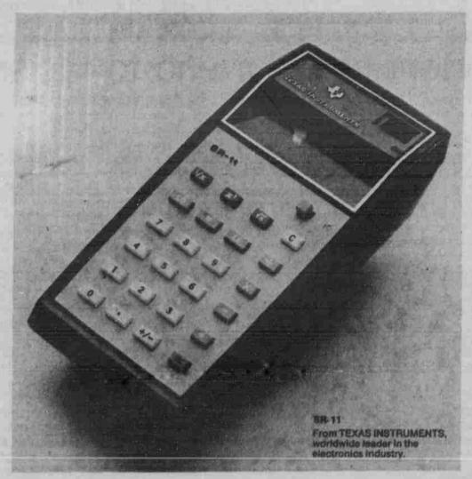
SR-11. A versatile, hand-held calculator with a range of nearly 200 decades (1090 to 10-08). Its capabilities include scientific notation (EE), square root (VX), reciprocals (1/x), squares (x2), change signs (+/-), plus mixed calculations, pi  $(\pi)$  as a constant and a constant for x, ÷. Data may be entered in free form (floating decimal, scientific notation or any combination of the two). Algebraic logic. Rechargeable. All accessories included. \$69.95
