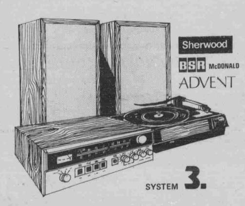
System 3 offers the Sherwood Stereo AM/FM Receiver, with significant refinements in bandwidth and distortion. The RMS power is 20 watts per channel at 8 ohms, or, more stringently measured, 17 watts per channel at 8 ohms, 40-20,000 Hz with Harmonic and IM distortion at 0.9%. The Sherwood S7110 comes complete with walnut-grain case.
