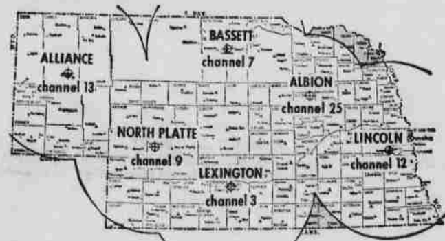
ETV—The above map shows Nebraska's proposed six-station ETV network. Shaded areas indicate supplemental translators service to provide total statewide ETV coverage.
