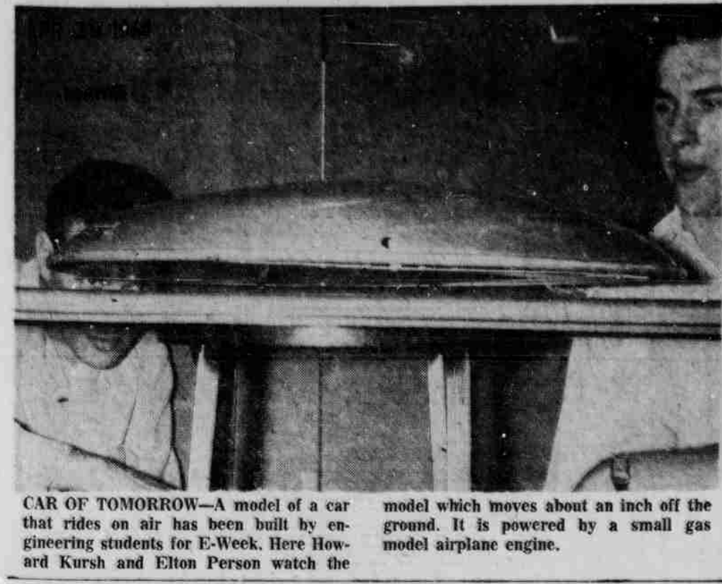
CAR OF TOMORROW—A model of a car that rides on air has been built by engineering students for E-Week. Here Howard Kursh and Elton Person watch the model which moves about an inch off the ground. It is powered by a small gas model airplane engine.
