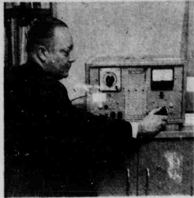
GET SET — Ed Simpson, University public health engineer, sets his Internal Proportional Counter for measuring radioactivity contained in dust from a University laboratory.
