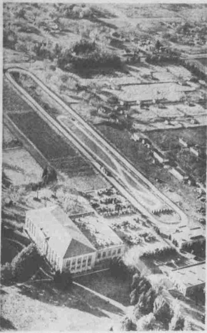
CENTER OF AG E ACTIVITY—The building to the left is the Ag Engineering building located at the north end of Ag campus. The long track is the tractor testing course and at the end of the track is the tractor testing lab. The lab is the only one of its kind in the world, and all tractors sold in Nebraska must be tested here first by state law.
