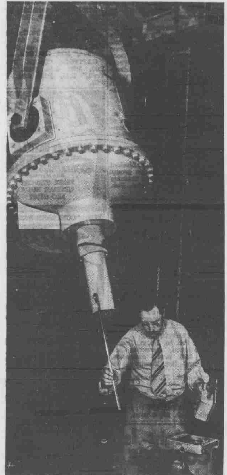
This 1,000,000-volt X-ray machine in Harvester's Manufacturing Research Department "looks through" 5½ inches of steel to examine the structure of fabricated parts. To protect operators and others from secondary radiation from its powerful tube, the machine is housed in a room with concrete walls 18 inches thick. Control is from a panel outside the room.
