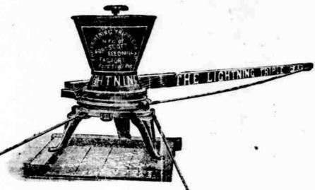
an hour with one horse. It has roller beorings, chilled steel burrs, friction plates to take up
