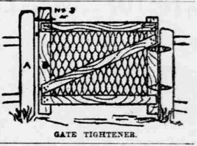
drawing it toward post A. In this way the gate can be made as tight as possible.
