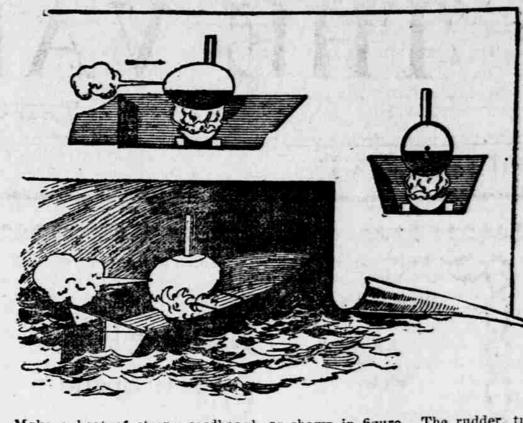
Make a boat of strong cardboard, as shown in figure. The rudder, turning about a pin as axle, is connected with the sides of the boat by two pieces of thread of uneven length, giving the rudder an angular position. A tub of water is the ocean on which our little boat will steam about.
