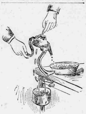
deposits the peas and pods in separate receptacles. The sheller is operated with a crank, and is mounted on an arm that can be clamped to a kitchen table, as shown in the illustration. The whole thing is not over seven inches high. It is made of galvanized iron and can be washed without injury to the parts.-New York Tribune.
