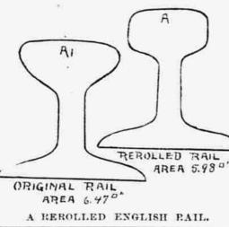
in the usual way, and after being cut to the desired lengths, were put on the hot bed to cool, subsequently being coldstraightened and drilled for splice bolts. The loss in heating and rolling ran from .05 per cent. to .08 per cent. With one heating furnace the product was over 100 tons per turn. A plant is being built at Joliet, Ill., to renew rails by this process.
