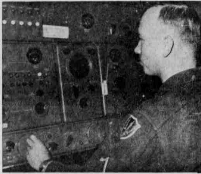
Pfc. Clinton E. Strouse of Genoa, Ill., checks a missile track radar console.
