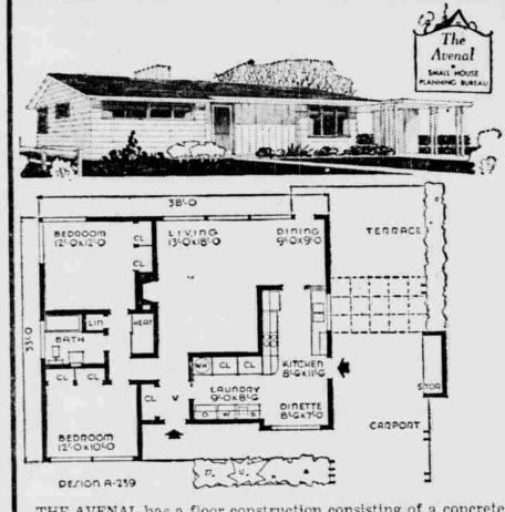
slab laid over a gravel or cinder bed and the superstructure is frame with wide siding, asphalt shingles and vertical siding in front recess and on storage room walls.
