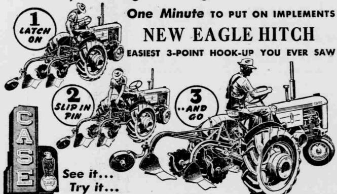
The new Eagle Hitch on the 1950 Case "VAC" tractor takes hold of the new latchon implements and picks them up-fast and easy. Without getting off the seat you just latch on, slip in a pin, and go! You get to the field quicker, finish sooner. Work is done better because the Eagle Hitch keeps implements working at a steady depth in spite of
