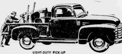
Model 3104-116-inch wheelbase, Maximum G.V.W. 4,600 lb. Other models available: 3604-1251/4-inch wheelbase, Maximum G.V.W. 5,800 lb; 3804-137-inch wheelbase, Maximum G.Y.W. 6,700 lbs
