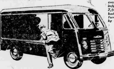
FORWARD-CONTROL CHASSIS More Chevrolet Trucks Model 39:42-137-inch wheelbase; in use than any other make Maximum G.V.W. 10,000 lb. Also available in model 3742-1251/4+ inch wheelbase, Maximum G.V.W. 7,,000 lb. Package Delivery type bodies suitable for mounting on the Forward-Control Chassis are supplied by many reputable manufacturer
