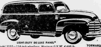
Model 3105-116-inch wheelbase, Maximum G.V.W. 4,600 lb. Also available in Medium-Duty model 3805—137-inch wheelbase, Maximum G.V.W. 6,700 lb.
