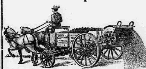
Is made of Oak, Malleable Iron and Steel with endless apron running on three sets of rollers which make it the easiest running and longest lit d spreader made. Notice the strong construction and practical lines followed in its building. Sold with either wood or steel wheels
