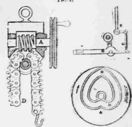
Above are given illustrations of three machine movements, which netted their originators fortunes. This is especially true of the worm and chain gear. mechanism for disengaging the eccentrie rod, A. from the valve rod, D. is shown, as is also an ordinary groove heart cam. Inventors and others desiring information as to inventions and oatent, should address Sues & Co., patent experts, Rec Building, Omaha. Neb.
