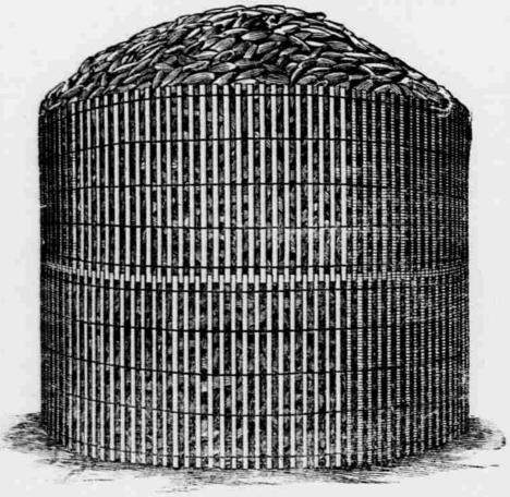
Made from No. 1 Yellow Pine 5% in. thick and 11/2 in. wide, 4 ft. long, all being bound together by machinery, by 5 double strands of No. 121/2 galvanized steel wire, and put up in rolls of five rods each. After filling up a crib 4 ft. high, place another length of 4 ft. on top of same, as shown in cut above. Thus we will have 10 cables of No. 121/2 galvanized steel wire holding together solidly our crib.
