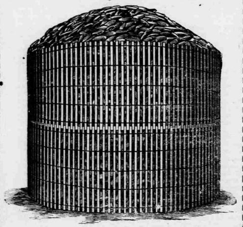
Made from No. 1 Yellow Pine & in. thick and 11 in. wide, 4 ft. long, all being bound together by machinery, by 5 double strands of No. 121 galvanized steel wire, and put up in rolls of five rods each. After filling up a crib 4 ft. high, place another length of 4 ft. on top of same, as shown in cut above. Thus we will have 10 cables of No. 121 galvanized steel wire holding together solidly our crib.
