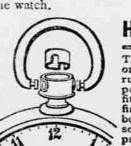
Here's the idea The bow has a groove on each end. A collar runs down inside the pendant (stem) and fits into the grooves, firmly locking the bow to the pendant, so that it cannot be pulled or twisted off.
