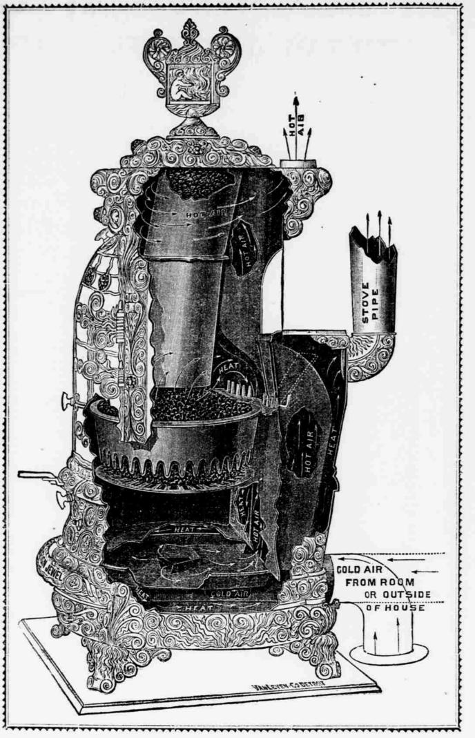
Air entering hot air flue at a temperature of 80 deg. is discharged at top at a temperature of 550 deg. This has been demonstrated by actual tests. Sovereign Jewel will heat 1/3 more space, with same amount of fuel, THAN ANY OTHER STOVE OF SAME SIZE. It is elegantly mounted and costs no more than any other First Class BASE BURNER in the market.
