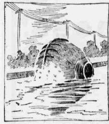
In this strange craft its French inventor has created a boat of remarkable appearance, if nothing more. It consists of two drums, the outer acting as a propellor, while the inner one contains a twenty-four horse power motor and carries the passengers.
