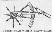
face of the wheel as pressure is exerted on the level. The device will fit any diameter of wheel by loosening the cams which connect the arms with the hooks, and adjusting the latter at the proper length. By placing the hook appointing. The new wheat has been ends on the ground and the end of the grown, except experimentally, in but lever beneath the axle this device can also be used as a wagon jack to recarry.
