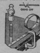
chanics. Center-punch the spring just hard enough to cause a bump at the point where the hole is wanted. Then grind off the protrusion. The operation must be repeated until the hole is the diameter desired. The method may be used on metal up to about 1/16" thick. Be careful, the magazine points out, not to strike the punch too hard. That might cause the steel to break or crack.
